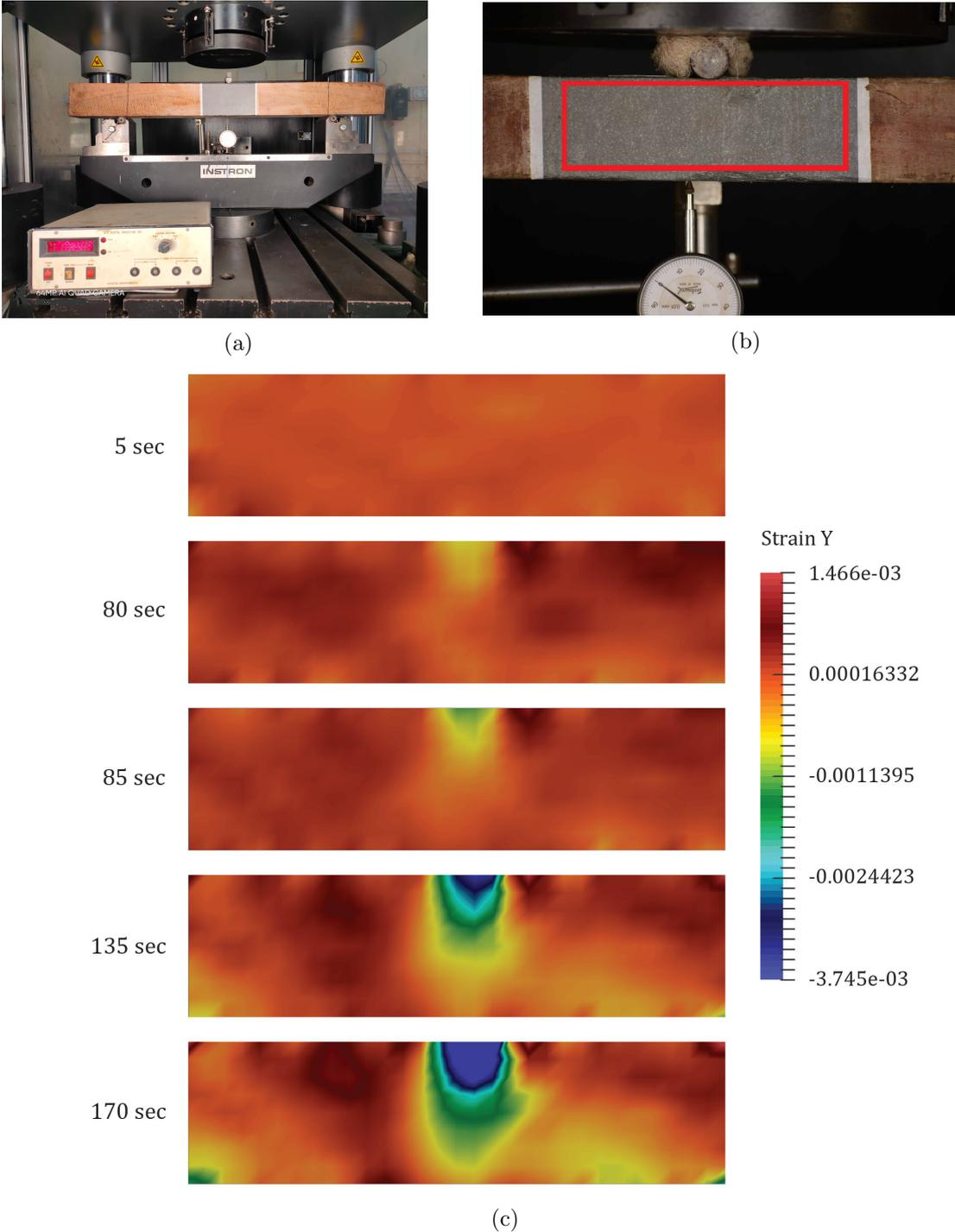
Figure 4: Three Point Bending Test
