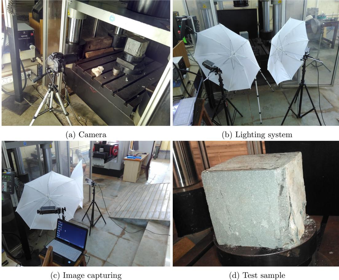
Figure 2: DIC setup developed in Rock Mechanics Lab
